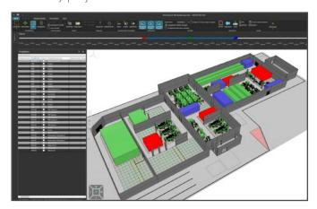
The integrated, immediate restriction check prevents multiple space allocations and thus costly planning errors. Any necessary rescheduling, extensions or development of new halls can be planned, tested and visualized directly in the tool. As a result, you reduce the planning effort, achieve greater planning and investment security and increase the capacity of your factory.
