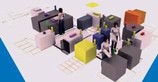
With VISUAL COMPONENTS, Faurecia is able to make models of schematic factory layouts and detailed production lines. To generate the simulation models, users select pre-existing components from the available libraries or create their own custom components. Statistical analysis gives an accurate evaluation of the planned process or layout in terms of performance metrics, such as: resource utilization or possible bottleneck areas.
